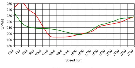
—— full load curve —— propeller curve
