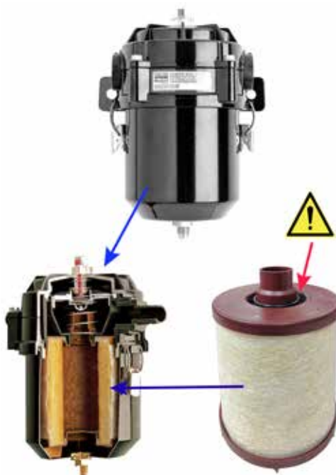
Crankcase assembly, cut away and filter views:
