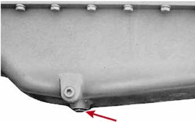
Above picture: pan draining oil - close up.
