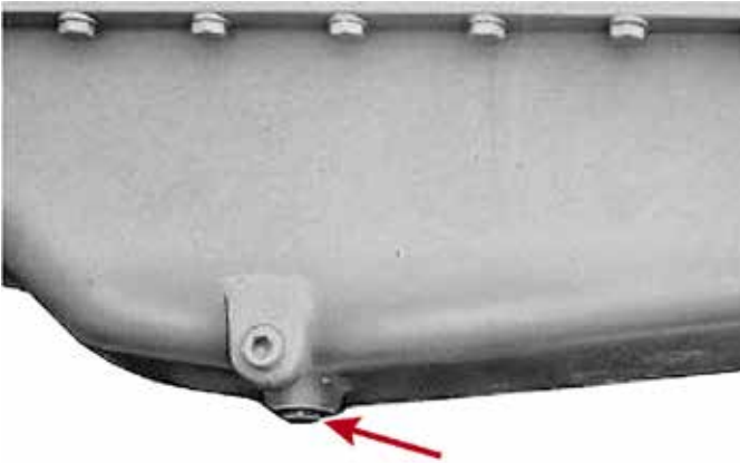
Above picture: pan draining oil - close up.
