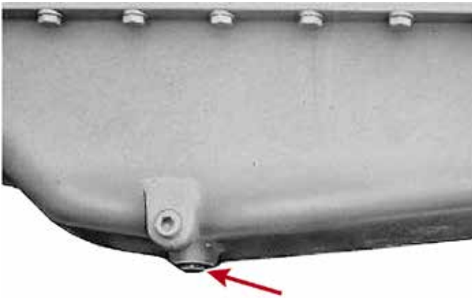
Above picture: pan draining oil - close up.
