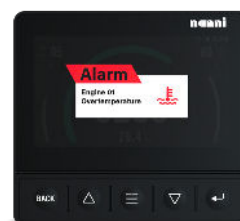
Warning / Alarm display
